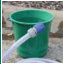
Step 1: Attach the One-Touch Hose Joint to one end of a 3 metre length of garden hose
