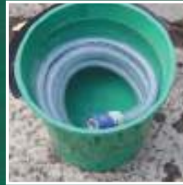
Step 2: Sink the entire 3 metre length of garden hose into a bucket filled with water
