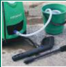
Step 4: Connect the washer to the power supply & switch on without the spray nozzle attached
