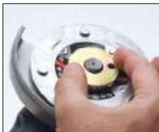
Use your standard locking nut to fasten the backing plate in place.
