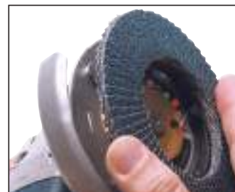
Match the CMT "loading" to the backing plate.
